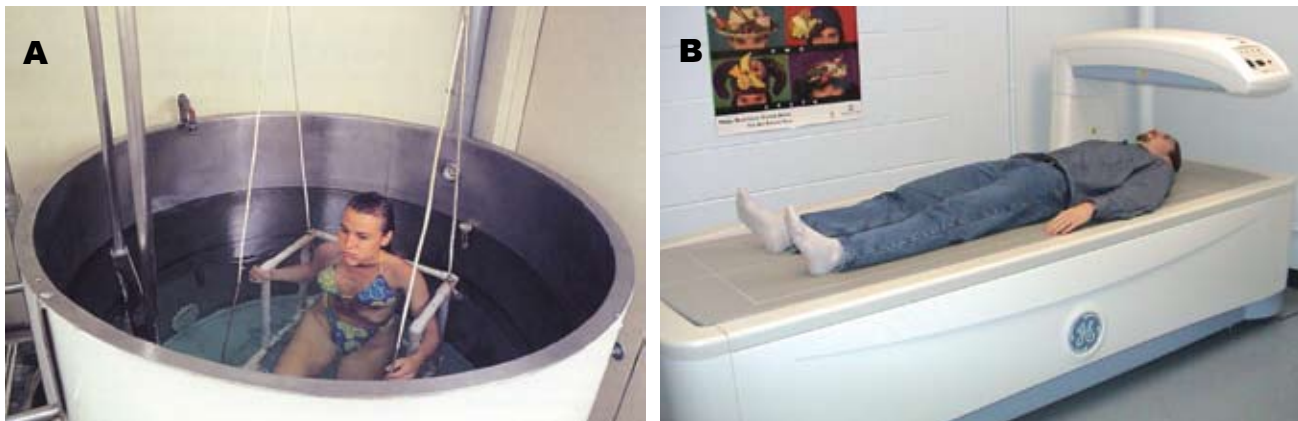
Figure 17.4 Research methods for establishing percent body fat. A. Hydrostatic weighing. B. Dual energy x-ray absorptiometry (DEXA).
